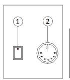
When the unit is turned on with the main on/off switch, and the temperature is set with analog thermostat to desired level, it takes about 20 minutes to reach the temperature.
